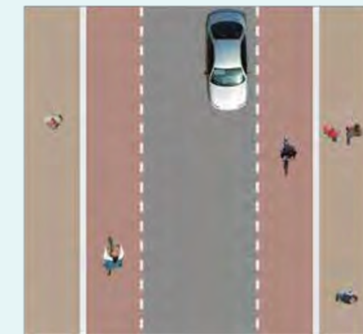
Plan view of proposed "Cycle Street" treatments on Quiet Streets (centre line removal)
