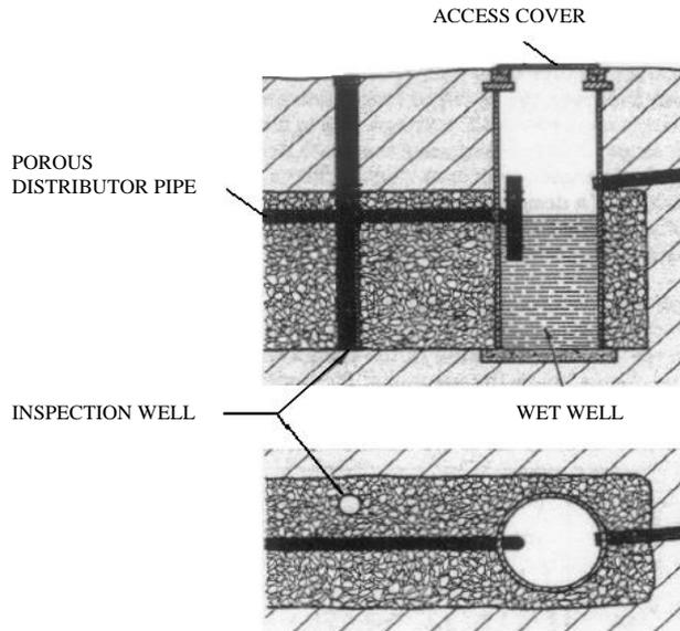
**Fig 5** Trench-type soakaway with large wet well equipped with T-piece overflow to porous distributor pipe and separate inspection well
