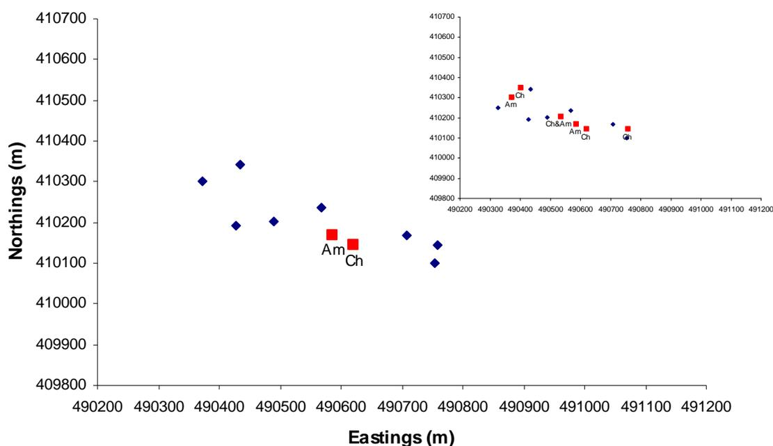
**Figure 3-1: spatial distribution of samples of near-surface soils/capping materials ( $\leq 0.5$  mbgl) screened for asbestos at the POS. Samples identified as containing asbestos are in red and the type of asbestos is also indicated (Ch=Chrysotile, Am=Amosite). Samples in which no asbestos was recorded are in blue. Inset: soil samples taken at all depths at the POS.**
