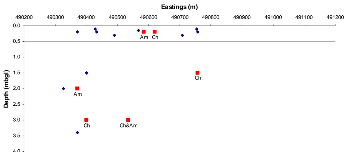
**Figure 3-2: depth profile along an east-west transect of all soil samples screened for asbestos at the POS. The mean depth of near-surface soils or capping material (0.5mbgl) is indicated. Samples identified as containing asbestos are in red and the type of asbestos is also indicated (Ch=Chrysotile, Am=Amosite). Samples testing negative are in blue.**
